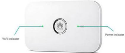
Huawei E5573 is a new 4G mobile hotspot with LTE Category 4 technology, so it can support the download speed to 150mbps and upload speed to 50mbps. On the front, there are two single LED indicators for battery and signal strength. The backcover of Huawei E5573 is removable, and it has external antenna connectors.
